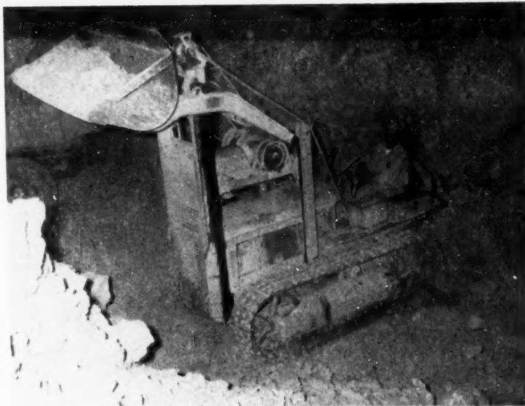
California scheelite miners were busy during night time in 1951 to better select and mine their ore indicated by ultra violet lights.
